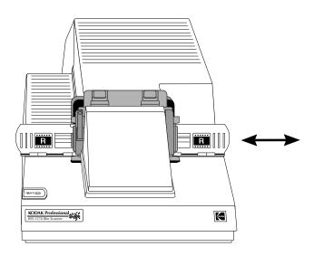
5. As you move the holder from side to side, you will feel it "drop" into place at each frame; this indicates that the holder is correctly positioned in the gate.
